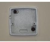
Next, plug the probe wire into the socket in the BACK of the face plate as shown below ensuring the neck of the plug sits in the aperture in the face plate (see below)
